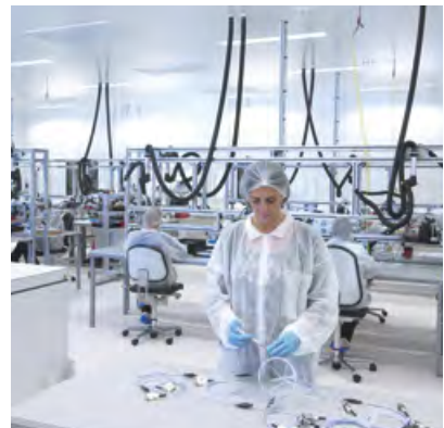
MANUFACTURE OF HARNESSSES IN ISO 8 CLEAN ROOM
